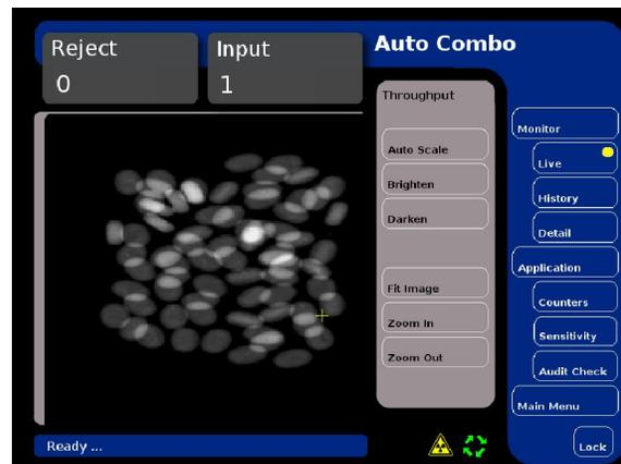
No key board or pointing device. All operations are accomplished with an intuitive touch screen interface which has no menu structure to learn or remember.
